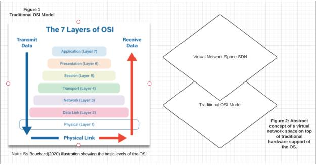
With the depreciated seven layer OSI model as a reference, we can see that SDN covers quite a few levels. Starting from the application and presentation layer, the iQuila software now carves out the Session layer, the Transport layer, the Network layer and the Data Link layer.
