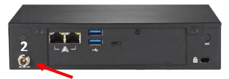
When ready attach the power supply to the E500 device (2).
