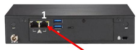
Plug in the Ethernet cable to your Internet into the WAN port (1) on the rear of the Bridge device
