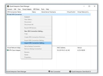
Navigate to where the config file was downloaded or stored. Select the file and click open. The file will setup a VEN Connection for that device based on information entered when the device was created. e.g. Host Name, Switch Name, Device Name, Password.
